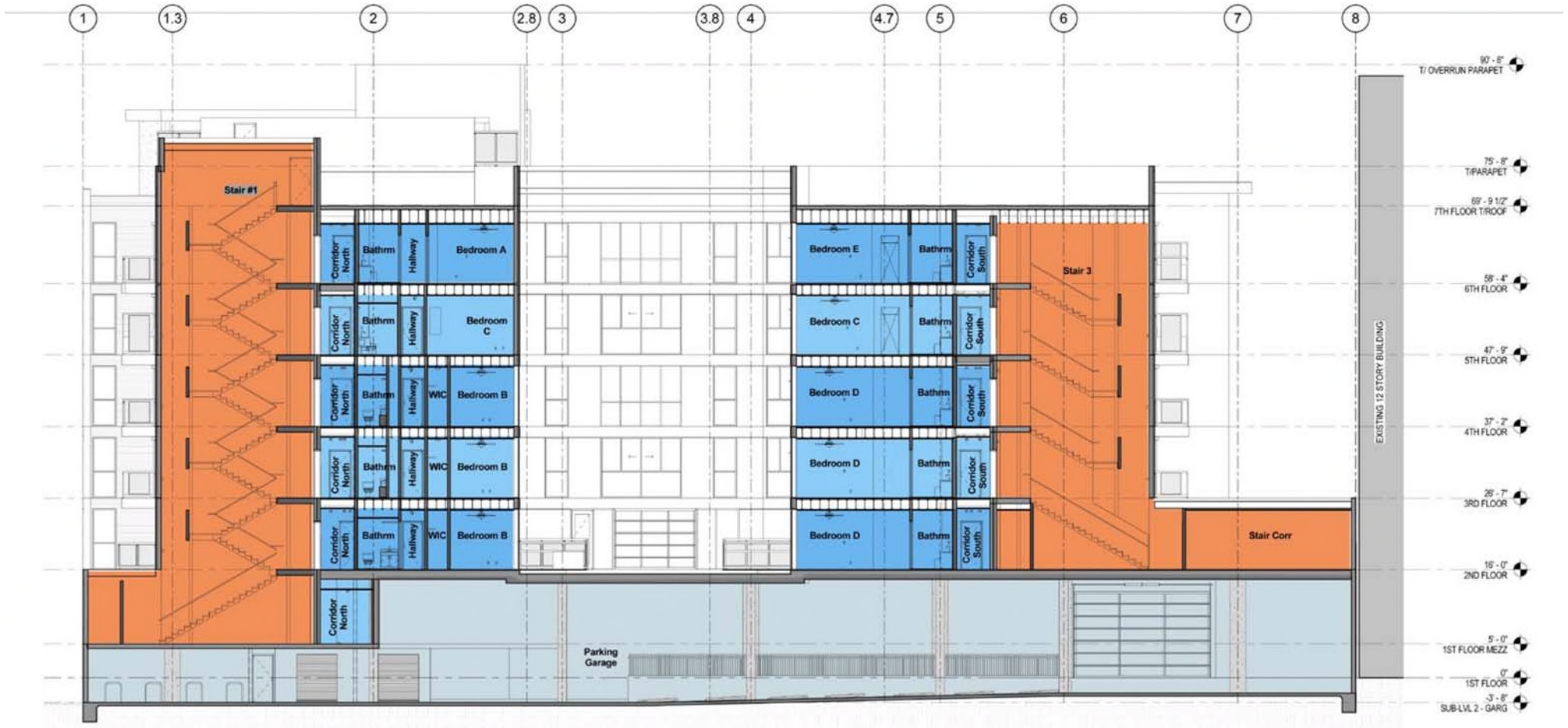
2 NORTH-SOUTH SECTION 2 - VIEW WEST SCALE: 1/8" = 1'-0"
