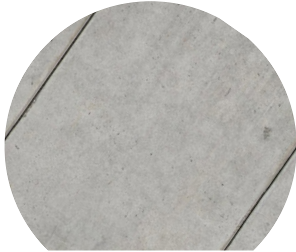
PAVEMENT-A INTEGRAL PEWETER BRUSHED CONCRETE
