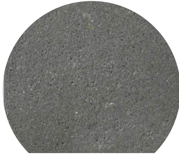
PAVEMENT-B INTEGRAL DARK GRAY EXPOSED AGG. CONCRETE
