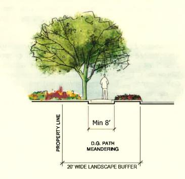
Figure 32: Perimeter Pathway Section
