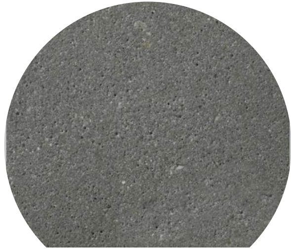
PAVEMENT-B INTEGRAL DARK GRAY EXPOSED AGG. CONCRETE
