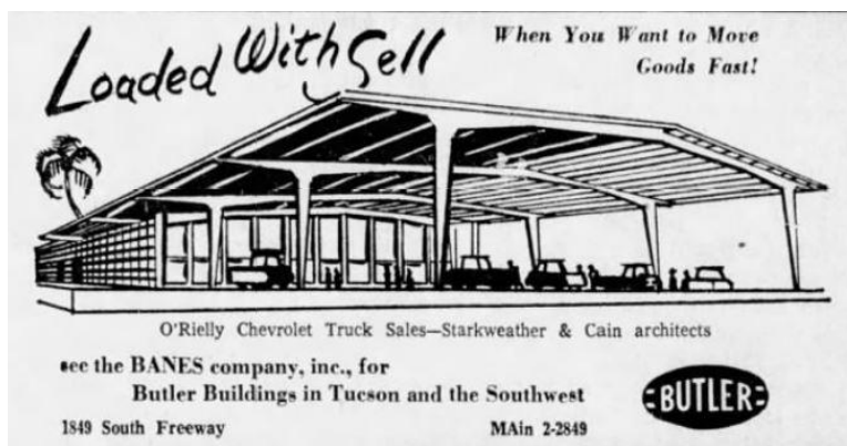
Figure 19. Newspaper advertisement for Butler Buildings showing the O’Rielly Chevrolet Truck Sales designed by Starkweather & Cain. Note the emphasis on structural components as ornament, the use of a window wall, and the textured block of the exterior walls, January 1961. (Courtesy of The Arizona Daily Star )
