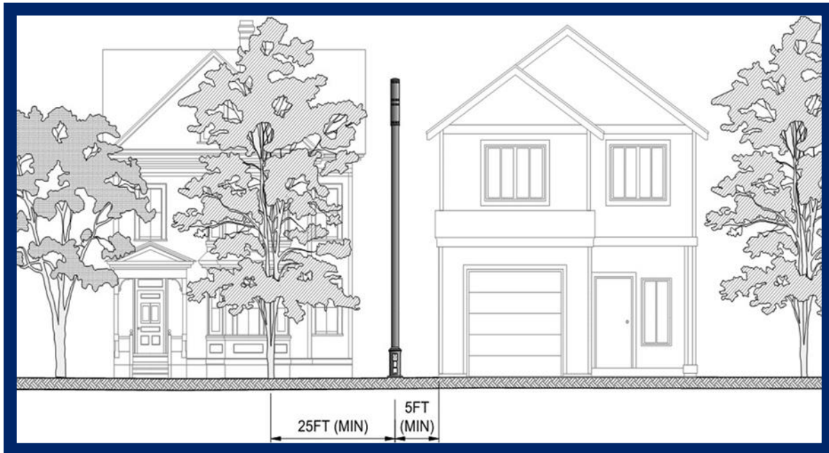
Figure 29: Separation from Driveways and Trees
