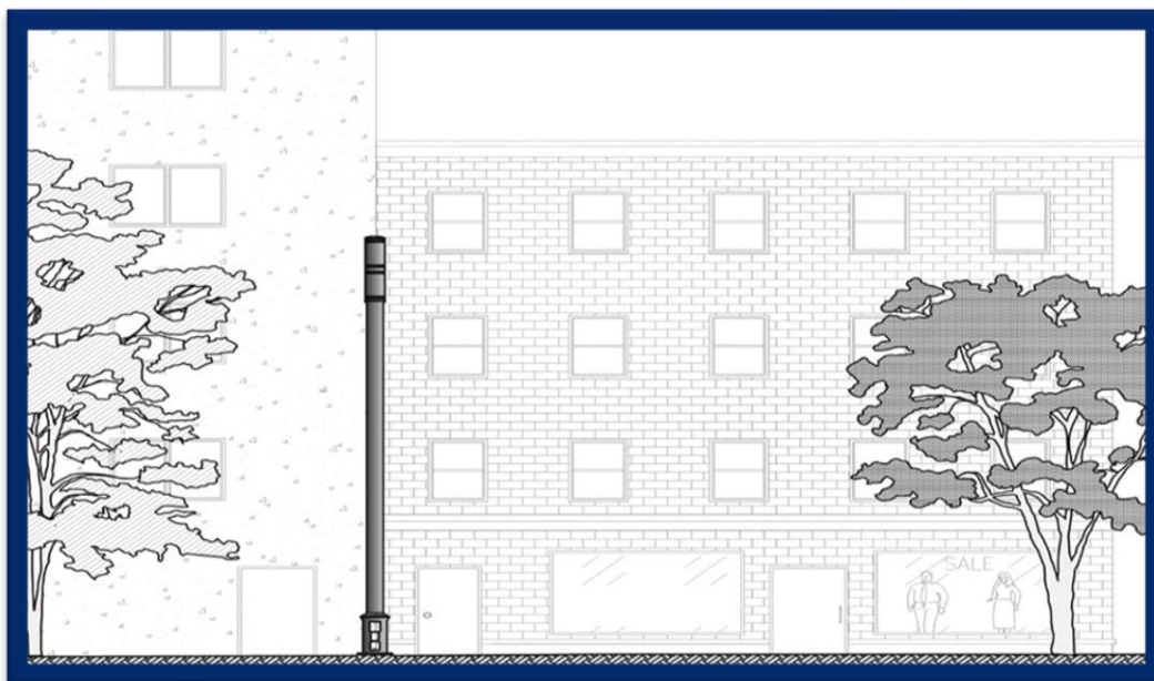
Figure 28: Pole Location at Common Property Line
