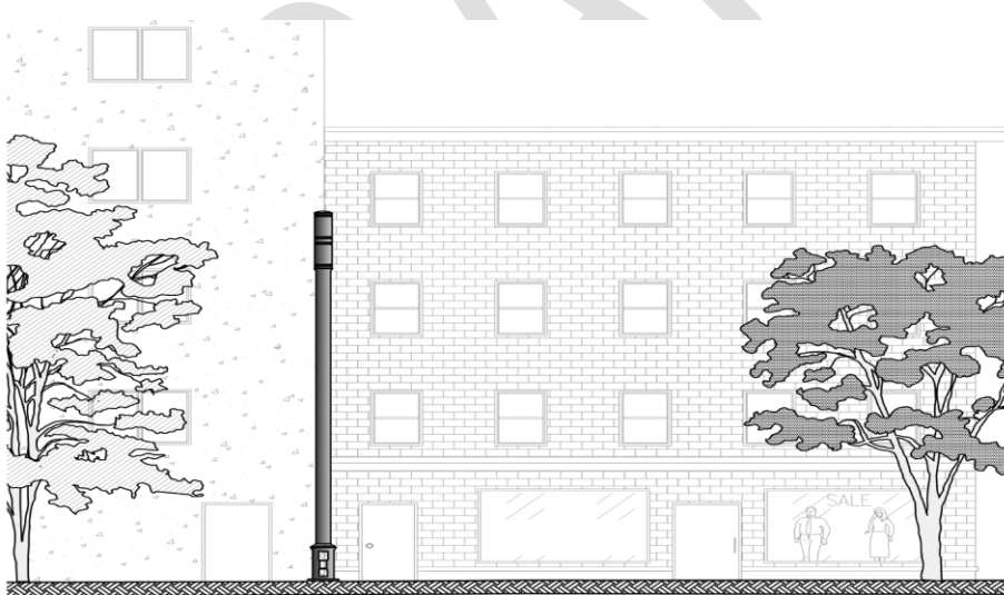
Figure 23 – Pole Location at Common Property Line
