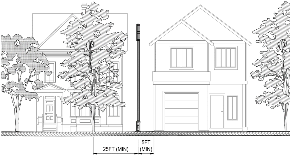
Figure 22 – Separations from Driveways and Trees
