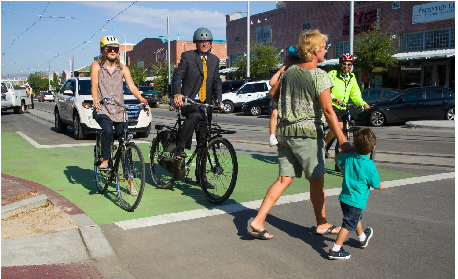
A bike box improves safety by positioning bicyclists in front of vehicles at the intersection of Park Avenue and University Boulevard. In 2015 approximately 3,410 bicyclists passed through this intersection each day.
