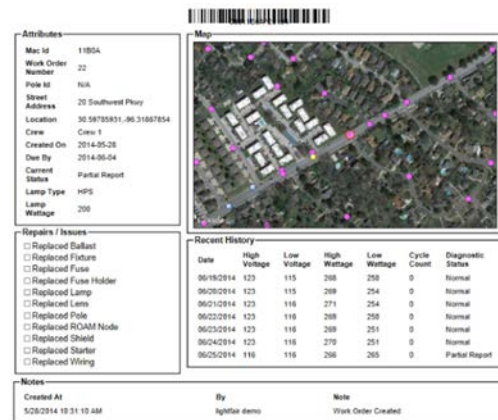
Figure D.13. ROAM Enterprise Customer Portal Work Order Management Module
