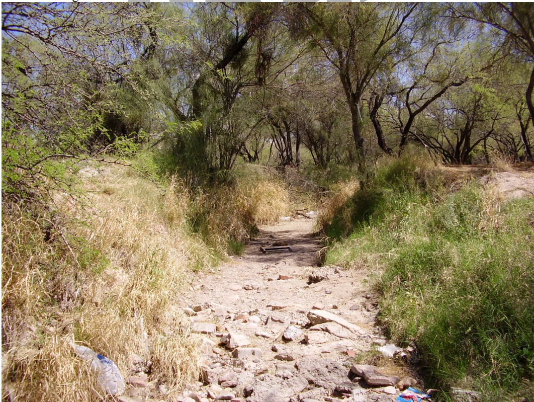
Rocky flow area, moderately dense bank vegetation, trees in banks, rough banks Channel Roughness = 0.050
